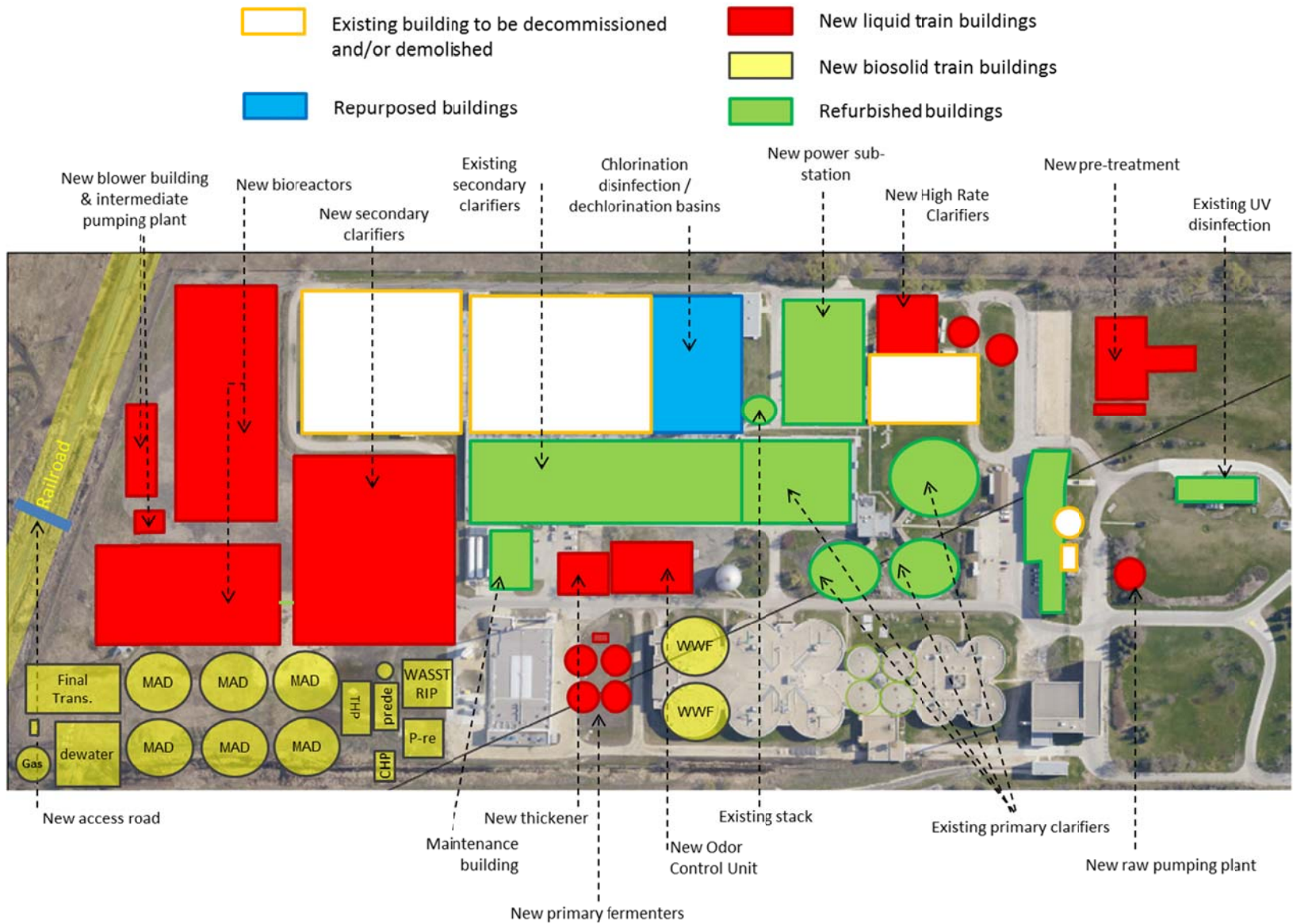
Figure 5.1 NEWPCC Upgrade Planning Layout
